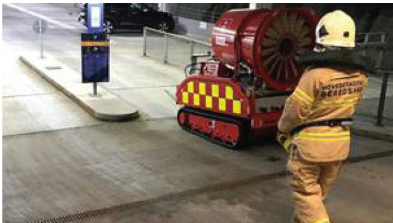
Use of LUF 60, respectively, for ventilation and towing of electric cars from parking garages or parking garages Photo: Hovedstadens Emergency Services
