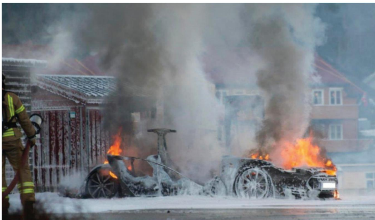
During a fire in a Tesla while charging on 1 January 2016 in Brokelandsheia in Norway, a fire broke out in the electric car's high-voltage battery. The fire lasted 23 hours and the car ended up being completely burnt out. After the extinguishing effort was over, there was still 400 V high voltage for approx. ¼ of the battery.
