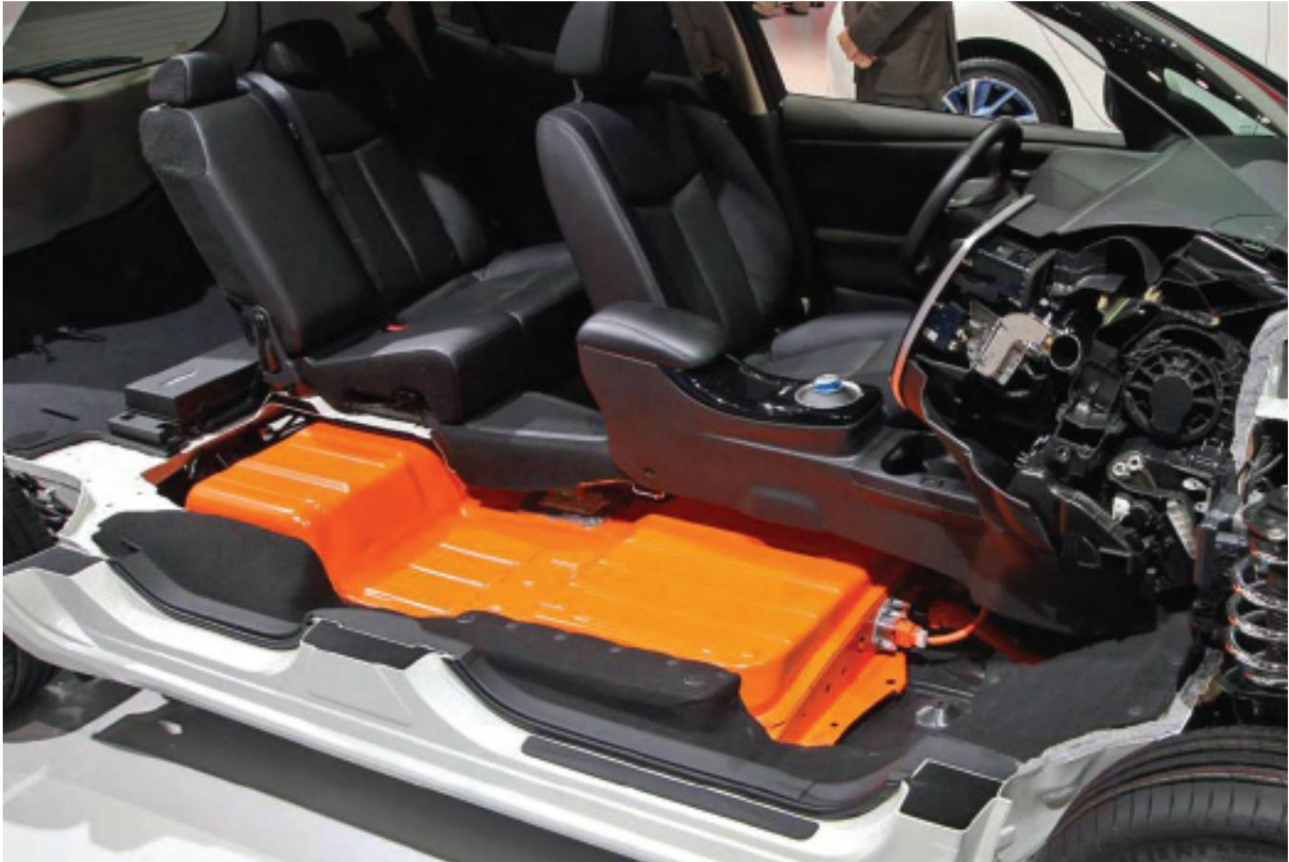
Battery frame integrated under seats in the cabin. Photo: Toyota
