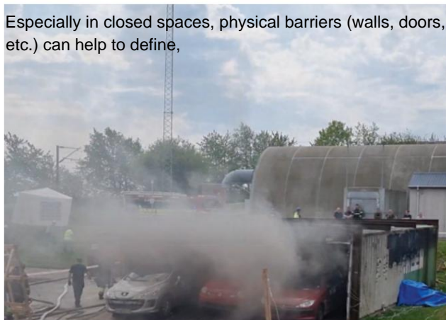
Photo 1: Fire in battery pack, the smoke is typically white with small brownish shades.
