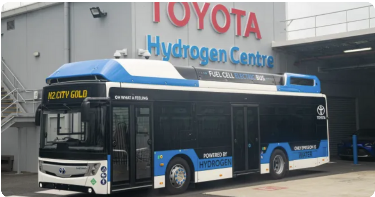
The H2 City Gold bus, built in collaboration by Toyota and CaetanoBus. This vehicles carries 37kg of Hydrogen gas and a lithium-ion battery pack, ranging from 44 - 80kWh. Ref: Thomson, 2022
