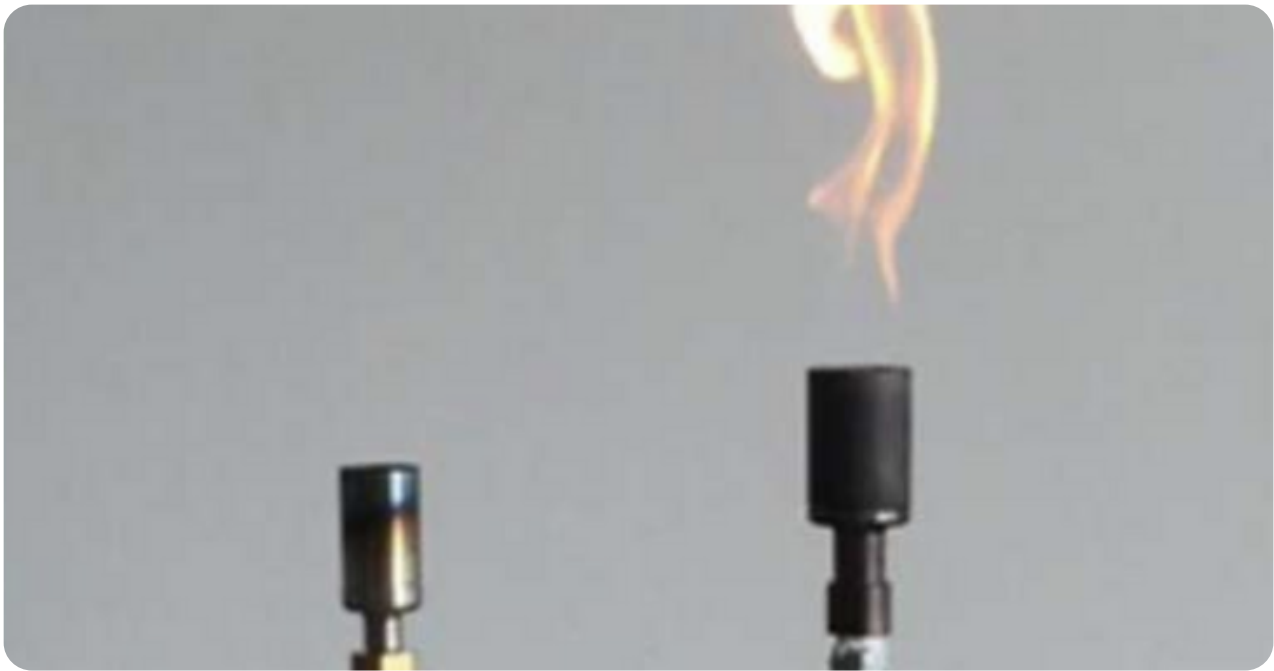
Hydrogen (left) burns with a invisible, more intense flame when compared to butane or propane gas (right).
