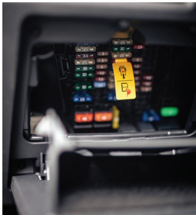
The two photos show the location of the main switch in an electric car model with two approaches to the switch - under the bonnet and behind the rear trim in the compartment to the left of the steering wheel.
