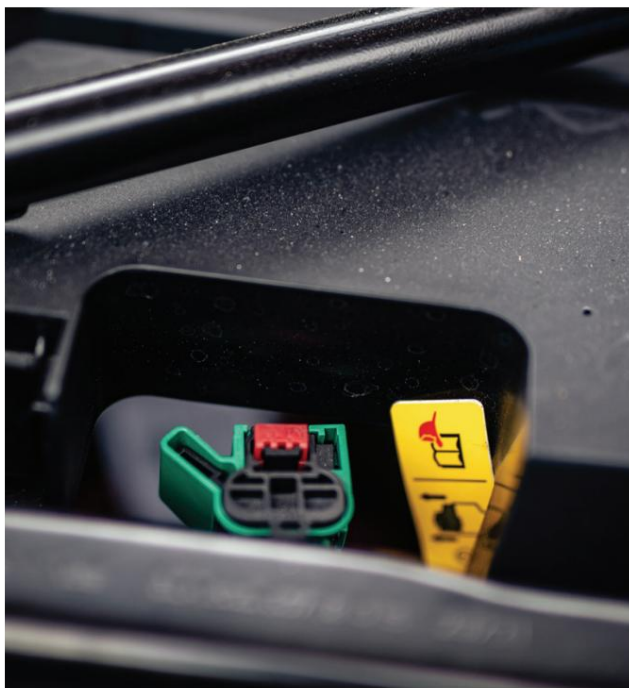
The two photos show the location of the main switch in an electric car model with two approaches to the switch - under the bonnet and behind the rear trim in the compartment to the left of the steering wheel.
