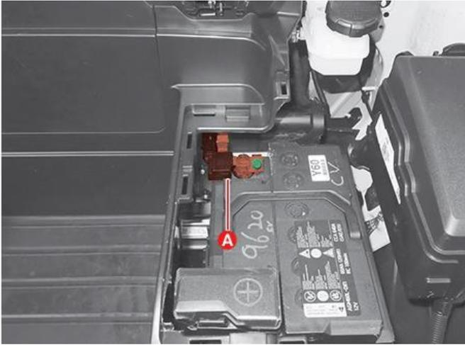
7. Pull up the yellow lever (interlock connector) to cut off the high voltage.
